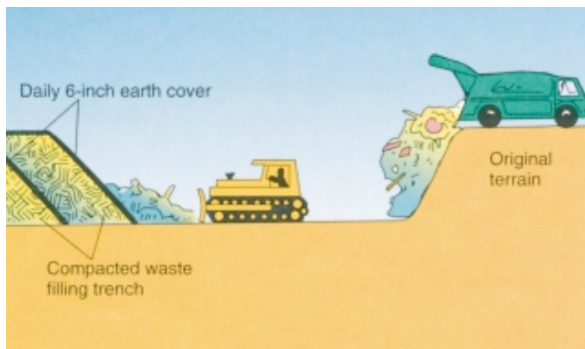
Figure 3.34 In a sanitary landfill, trash and garbage are crushed and covered each day to prevent accumulation of vermin and spread of disease. A waterproof lining is now required to prevent leaching of chemicals into ground water.
