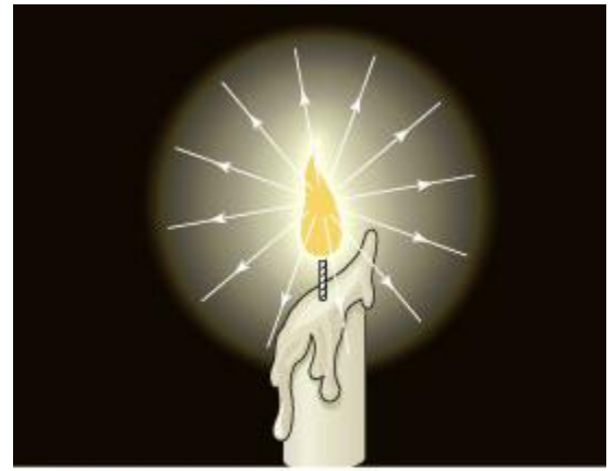
Figure 5.2 A ray is an imaginary line showing the direction in which light is travelling.
