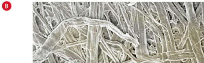
(B) Scanning electron micrograph of the surface of paper
