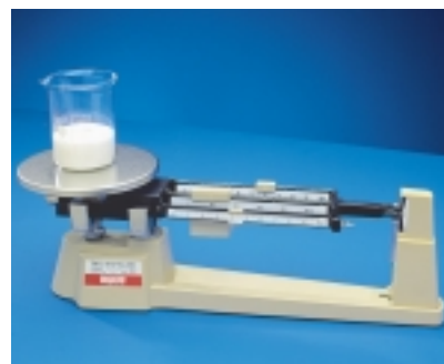
C Carefully add the solid to the beaker on the pan of the balance. The scales will be balanced again when 100 g of solid have been added to the beaker.
