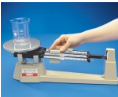
B Add 100 g to the mass measurement by moving the appropriate rider along the beam.
